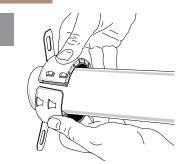
Flex collar open and wrap around pipe, anchor tabs to be facing mounting surface
