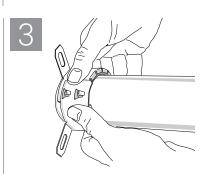
Press slots down and back (towards mounting surface) over hooks and lock into the closed position.
