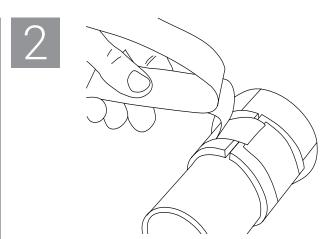
Secure wrap strip in place using foil tape.
