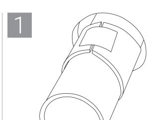
Tightly apply wrap strip around pipe/tube with ends of wrap strip tightly butted. See appropriate UL System for required number of Wrap Strip Layers.
