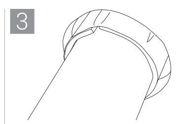
Slide wrap strip along pipe/tube into opening. See appropriate UL System for positioning requirements.
