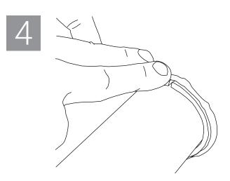
Apply SpecSeal® Firestop Sealant into annular space between wrap strip layer(s) and wall assembly. See UL System for acceptable Sealant types and sealant depth requirements.
