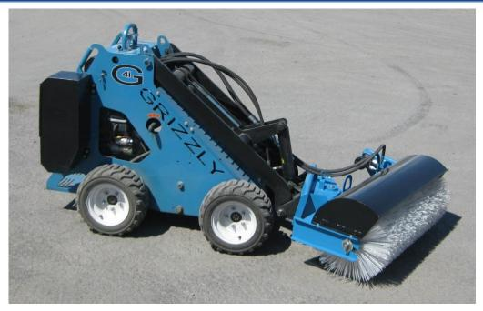
This 44" sweeper allows you to sweep forward, to the left or to the right depending on your needs. The brush rotation speed is adjustable. A high rotation speed will be used to throw debris and snow a fair distance or a slower speed will be used when keeping debris like stones and rubble closer to the brush is important.
