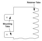
1.Temporarily secure wrap strips to pipe with masking tape. Measure and cut collar to length, providing a 1" (25 mm) overlap.
