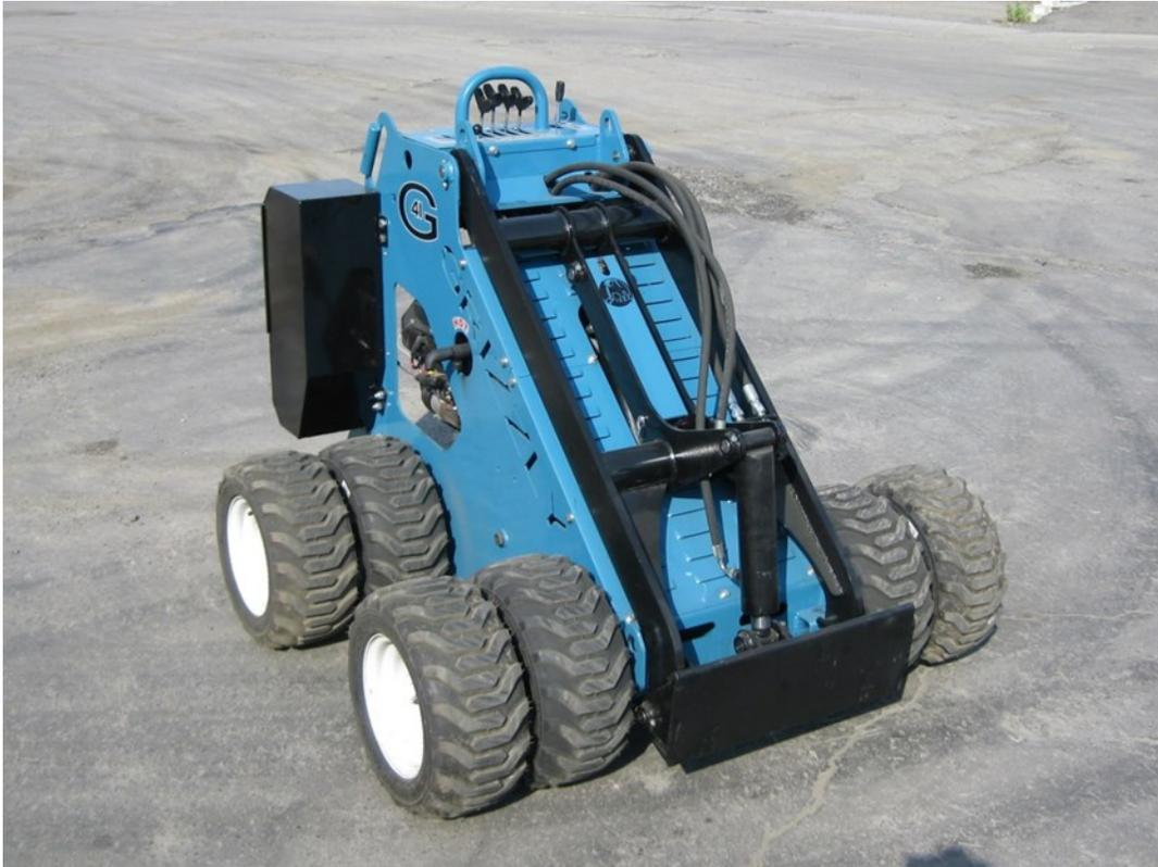
This dual wheel kit is EASY ON, EASY OFF! This simple option allows the weight of this already light machine to be spread over eight wheels allowing it to work over soft or fragile surfaces with more confidence. Operator is ultimately responsible for working on any surface and must proceed with care.
