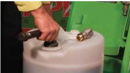
The vent fitting fits into the 2 inch opening to allow materials to flow smoothly. This is the larger of the two holes.
