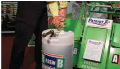
Point vents away from the Patriot Jr. in a horizontal position away from the cart so that when it's laying down the vents will face up.
