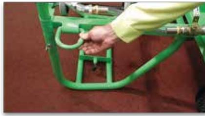
There are 4 lifting D-Rings on either side of the cart in each corner.
