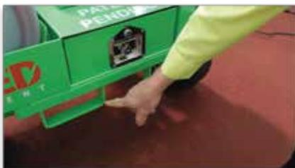
It Has forklift pockets for lifting the cart.
