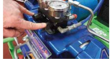
The recirculation controls are the two black switches on the top below the two round pressure gauges.
