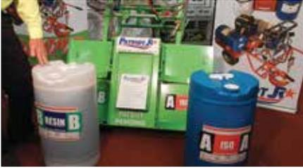
When installing the barrels on the Patriot Jr. be sure to first place the barrels on the correct side matching the A side and the B side.
