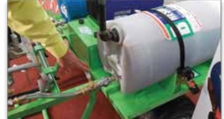
The A-Side has the same parts as the B-Side. These are the valves to turn on and off.
