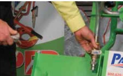
Make sure to note that this male plug goes into the female insert in the barrel for the B-Side barrel.
