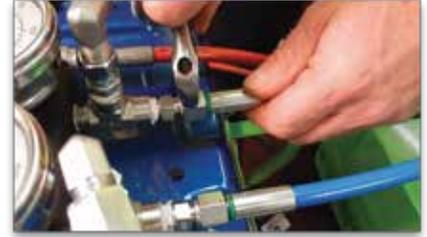
Be sure to carefully tighten each hose connection.
