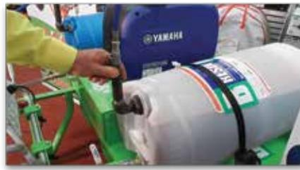
The silver tubes are the air vents for your drums (even though it is shown in black here).
