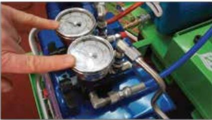
The pressure gauges show the pressure in your spray line.
