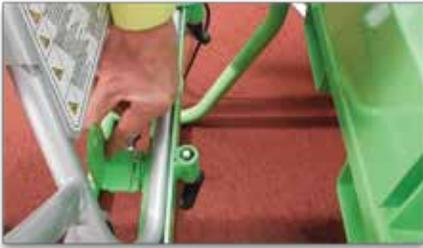
Make sure the clips are down and in place so that when you tilt your cart up the pump does not fall out. There are 2 clips in the back and one in the front center below with pressure gauges.
