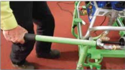
The handles are for lifting and maneuvering the cart and can be swung out of the way at the end of the night
