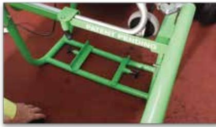
There are two clips on the bottom base to hold the air compressor. The typical gun uses an air gun so that is why you would need the air compressor.
