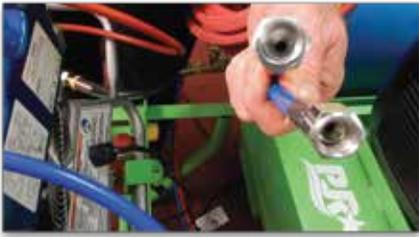
When hooking up the hoses to the PJR The hose diameter is the same but the fittings are different sizes so they can only go on one way.
