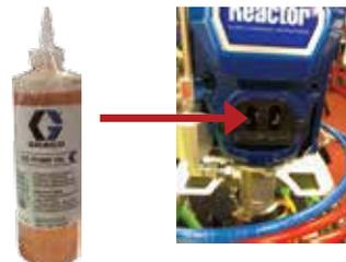
Squirt the provided ISO oil 1 time in the pump in the AM in BOTH ends of the reactor.
