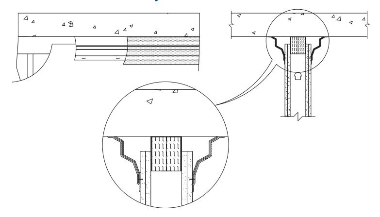
System Number HW-D-0846 is a NEW head-of-wall joint system for 1 or 2 hr fire-rated gypsum walls abutting concrete floor assemblies.
