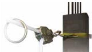
8. Attach complete and compatible PFAS to HLL O-ring. Maximum 1 connection per O-ring. Guardian Fall Protection snap hooks and carabiners may be directly connected to Guardian rope HLLs, however connecting to O-rings is considered best-practice use.
