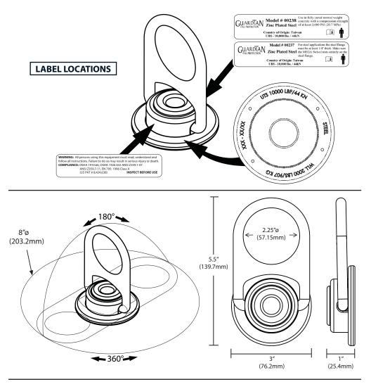
Tensile Strength (UTS): 10,000-lbf (44kN) Working Load: 2,000-lbs (907kg) Weight: 1.2-lbs (544.3g) Materials: Zinc Plated Steel Regulatory Compliance: Meets or exceeds ANSI Z359.1-2007, ANSI Z359.7-2011 OSHA 1926.502, OSHA 1910.66, EN 795:1996 Class A
