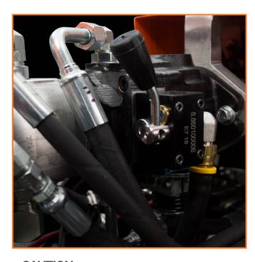
Freewheel Control Lever. Using valve pressure when engaged, this lever locks the wheels when the the machine is not in use. When opened, the machine may be moved without engine operation.
