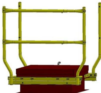
**STEP 5** — Attach front side mid and top rail assembly to upright using (A) 2-1/2" x 3/8"-16 Button-Head Cap Screws.
