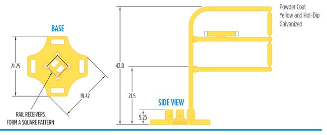
Roof Edge Protection: Provide freestanding pedestrian egress barrier system on roof, including pipe railings, uprights, bases, and fittings
